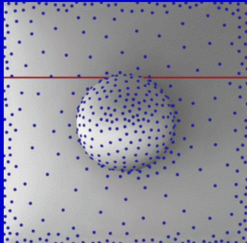
Figure 1. Blue dots show calculation points for diffuse interreflection.
